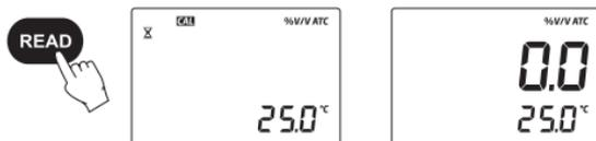
*Note: The last measurement value will be displayed until the next sample is measured or the instrument is turned off. Temperature will be continuously updated.*
