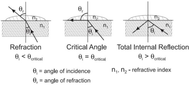
In the [HI96816](#), light from an LED passes through a prism in contact with the sample. An image sensor determines the critical angle at which the light is no longer refracted through the sample.
