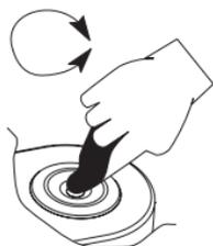
2. Using a plastic pipette, drip sample onto the prism surface. Fill the well completely.
