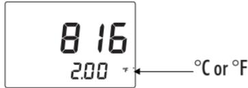
The %Brix value can be checked by pressing and holding the **READ** key, until the %Brix value on the primary LCD is shown.
