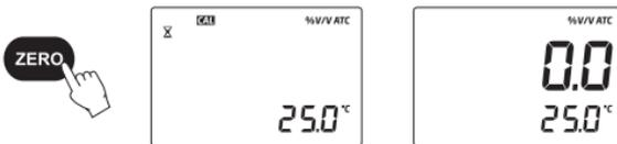
4. Gently absorb the ZERO water standard with a soft tissue. Use care not to scratch the prism surface. Dry the surface completely. The instrument is ready for sample measurement.
